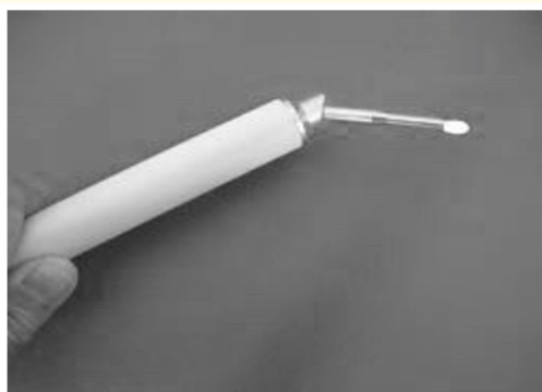
Figure 2: A probe to delivery microcurrent to specific acupuncture points.
